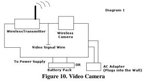
The Camera sees the image, the camera then provides the video to the transmitter, then the transmitter sends the wireless signal to the receiver. There are many types of wireless cameras. You can make most any camera wireless by adding a wireless transmitter and receiver. The camera and transmitter require power. The power is provided by battery and/ or transformer / adapter.
